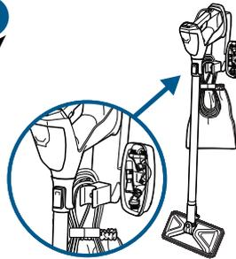
Store on the Wall Mount that is securely mounted to a wall in a protected, dry area. Store with dry pads as wet mop pads may damage wood and other delicate hard floors.
