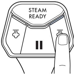
Push the HI STEAM button once to turn ON. Use HI STEAM when cleaning durable floors or sticky messes.
