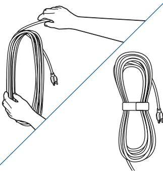
Wrap the cord around the palm of your hand into a circle. Then, place the wrap strap around the cord and back onto itself to secure.
